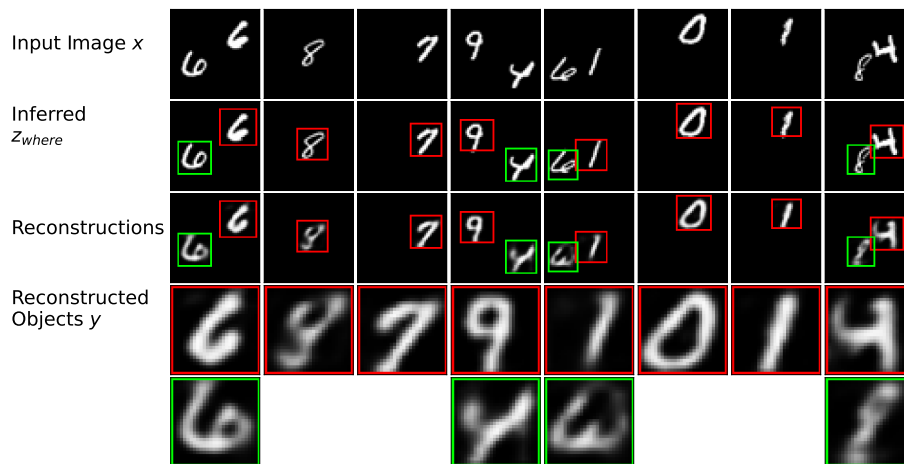
Figure 3.1.: AIR (Eslami et al., 2016) takes an input image x and infers object positions z_{\text{where}} in the form of bounding boxes. Their contents y are modeled via variational autoencoders, yielding a reconstruction of the overall scene. This figure was produced using the implementation by Bingham et al. (2018).
