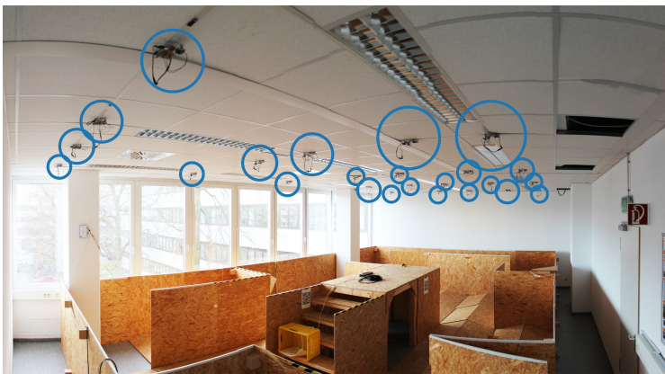
Figure 5.6.: Left: the RoboCup Rescue arena at the GKmM Lab, with 25 nodes on the ceiling (arrays #1 to #5). Right: fully assembled CM5000 (a TelosB clone) with adapter board for the external DS1000 set of CO/CO 2 /temperature sensors, attached to the USB and power infrastructure.
