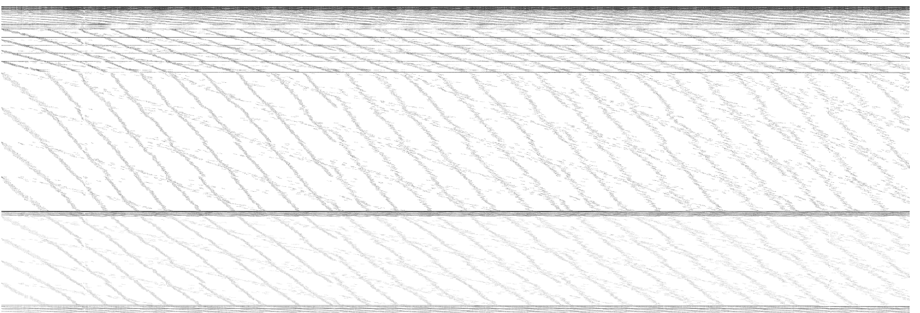
Figure 7.17: Trace C_d scatter diagram. The typical TPC-C blocktrace is depicted, showing only the accesses of the delivery relation.
