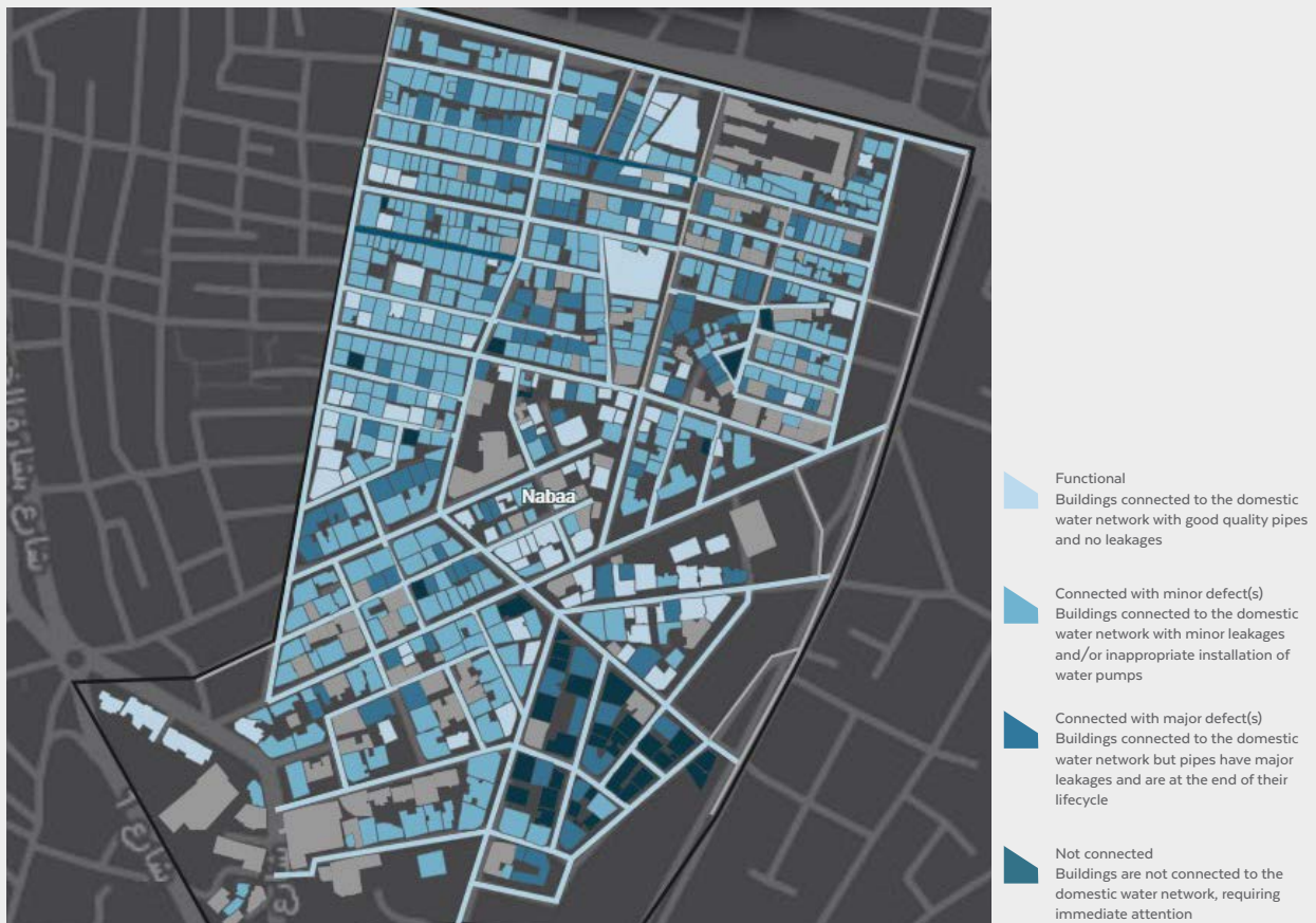
Figure 58 Condition of buildings’ connection to the network in Nabaa neighbourhood. Source: UN-Habitat and UNICEF, Nabaa Neighbourhood Profile 2017.
