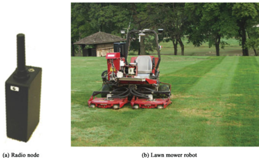
Figure 2. (a) The UWB radio nodes used in our work. (b) The autonomous lawn mower.
