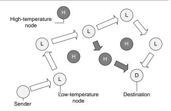
Fig. 6 An example of LTR and ALTR. The white arrows indicate the LTR-path. The shaded arrows show the adapted path of ALTR. When the path has three hops, the routing algorithm switches to shortest path routing.
