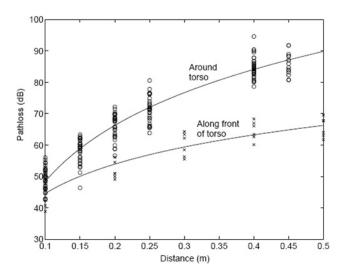
Fig. 5 Measured path loss versus the distance around (NLOS) and along the torso (LOS). It can be clearly seen that line-of sight communication experiences a lower path loss [58].
