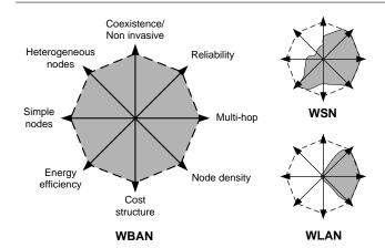
Fig. 4 Characteristics of a Wireless Body Area Network compared with Wireless Sensor Networks (WSN) and Wireless Local Area Network (WLAN). Based on [44].
