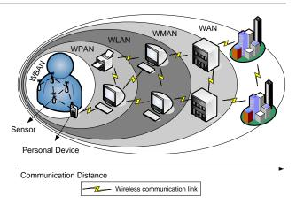
Fig. 3 Positioning of a Wireless Body Area Network in the realm of wireless networks.
