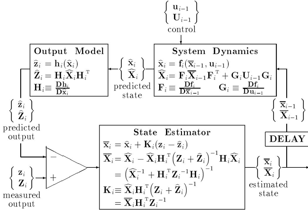
Figure 5: The Extended Kalman Filter equations.
