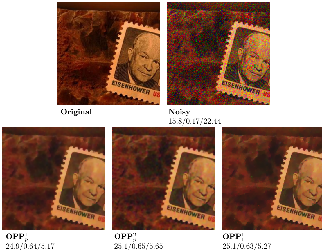
Figure 7.6: Example result images from the evaluation dataset for 60 standard deviations of noise. \text{OPP}_p^2 performs well in images with piece-wise affine regions as indicated by the high SSIM value, although with respect to color consistency \text{OPP}_1^1 shows marginally better result. (PSNR/SSIM/CIEDE)
