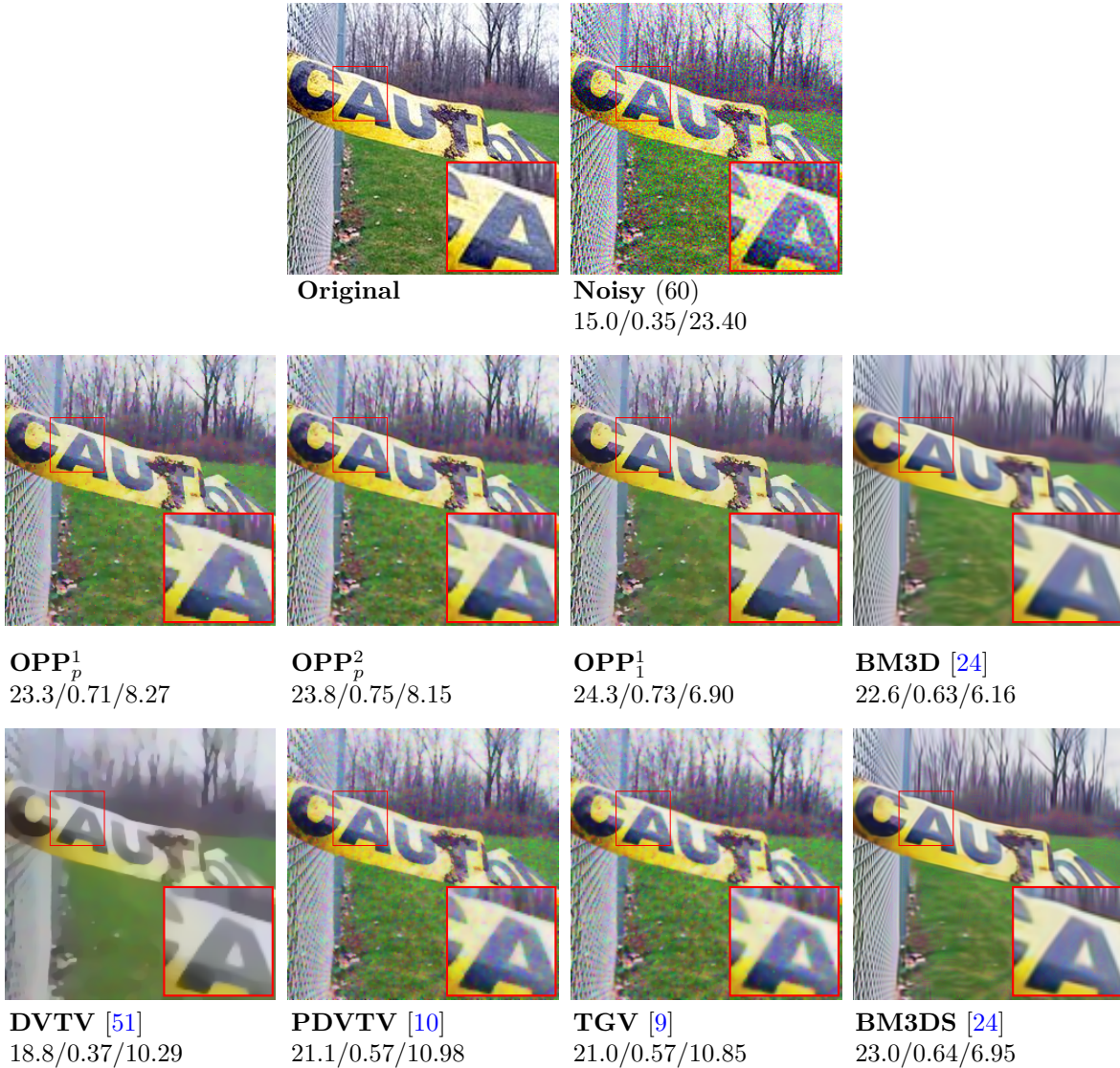
Figure 7.3: Visual comparison of the compared methods and corresponding error values. The result of our OVTV produces the most accurate result, only marginally beaten by BM3D in terms of color accuracy. Yet, the visual quality of OVTV is more clear and does not suffer from desaturated colors as in DTV.
