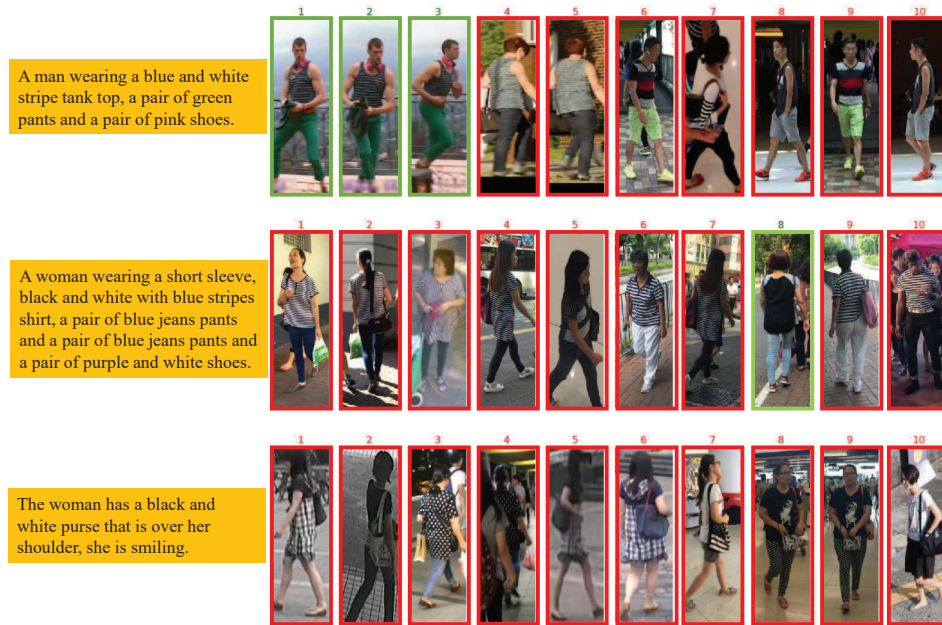
Figure 5: Qualitative image search results using text query by our proposed DCMG. The results are sorted from left to right according to their confidence. The images in green boxes are the true matches, and the images in red boxes are the false matches. Successful searches (Rows 1-2) where corresponding persons are in the top-10 results. Failure cases (Row 3) where corresponding persons are not in the top-10 results.
