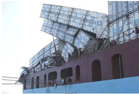
Figure 1.8: Unbalanced yard-bay at one vessel.
