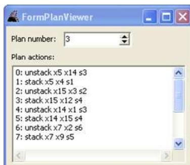
Figure 2.5: The obtained plan solution to be carried out by the transfer crane.
