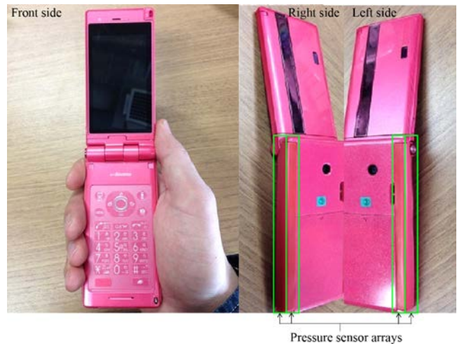
Figure 1. Experimental mobile phone with pressure sensors.
