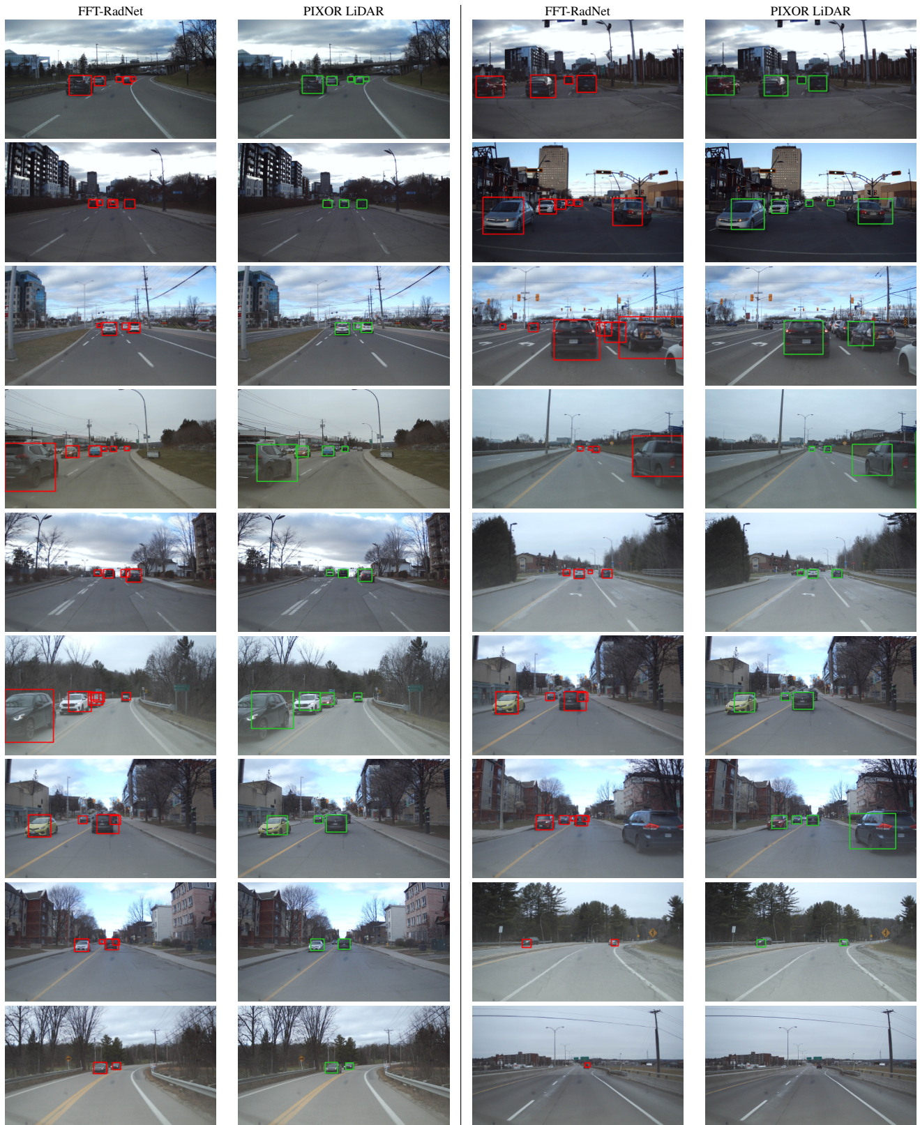
Figure 7. Examples of vehicle detection in complex scenes using either HD radar or LiDAR. Comparison between Pixor trained with LiDAR point clouds (‘PIXOR LiDAR’ columns, green boxes) and our proposed FFT-RadNet requiring only range-Doppler as input (‘FFT-RadNet’, red boxes). Note that radar detections are not limited to the first row of vehicles but can see up to the second one. Also, FFT-RadNet provides vehicles’ relative speed through Doppler measurements.
