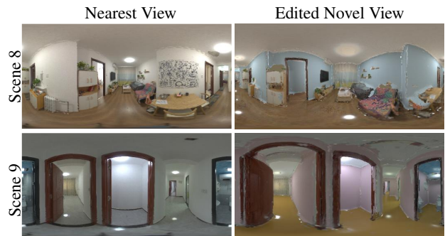
Figure 10. Editable novel view synthesis. In Scene 8, we edit the albedo of the wall, and edit the roughness of the floor. In Scene 9, we edit the albedo of the floor and the wall. Our method produces convincing results (see the lighting effects in the floor and wall).
