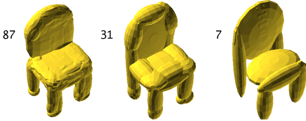
Figure 12. Shape abstraction levels. A chair in CADTalk-Ellip with different numbers of ellipsoids.
