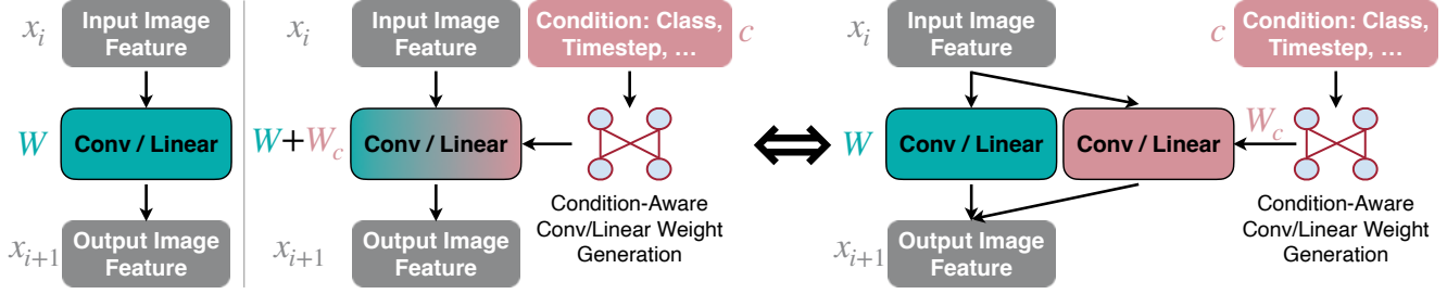
Figure 2. Illustration of Condition-Aware Neural Network. Left: A regular neural network with static convolution/linear layers. Right: A condition-aware neural network and its equivalent form.
