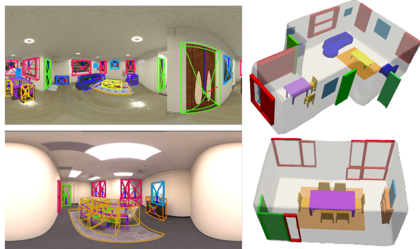
Figure 1. Given a single RGB panorama, we simultaneously estimate the room layout, oriented object bounding boxes (left), and full scene meshes (right). The first and second rows are examples from the iGibson-Synthetic [57] and ReplicaPano datasets.
