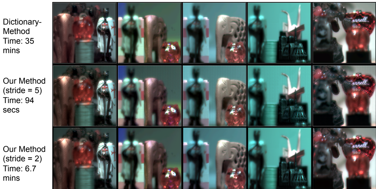
Figure 8. Real ASP Data: We show the reconstructions for the real data from the ASP measurements using our method (for stride 5 and stride 2) and dictionary method (for stride 5), and the corresponding time taken. It is clear that the spatial resolution for our method is comparable as that using the dictionary learning method, and the time taken for our method (94 seconds) is an order less than that for the dictionary learning method (35 minutes).
