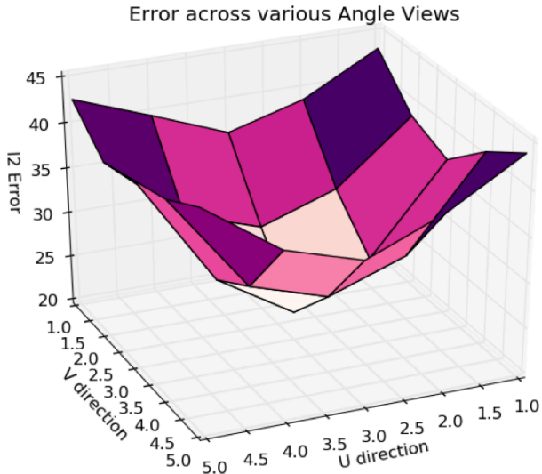
Figure 5. Error in Angular Viewpoints: Here we visualize the \ell_2 error for a light field reconstruction with respect to ground truth using a standard \ell_2 loss function for training. Notice how the extreme angular viewpoints contain the highest error. This helped motivate the use of a weighted \ell_2 function for training the network.
