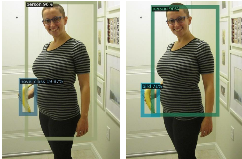
Figure 8. The left column shows the predictions in Task-1. The banana has not been introduced, the model has correctly predicted the novel categories. The right column shows the predictions in Task-2 where the food classes are not available for the task. The model should predict the banana into one of the novel categories, but it incorrectly classifies the unknown object into one of the known classes.
