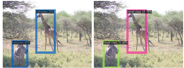
Figure 3. Comparison between OSOD and OSODD prediction. OSODD (Right figure) has extended the OSOD (Left figure) prediction by assigning novel category labels to instances of an unknown class.
