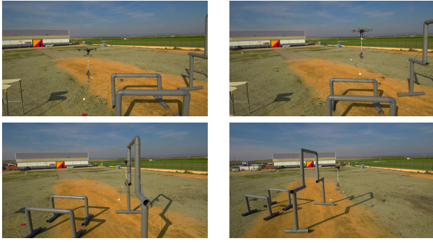
Fig. 9. Execution of the planned trajectory by the controlled ARS-LRM system. Experimental results.
