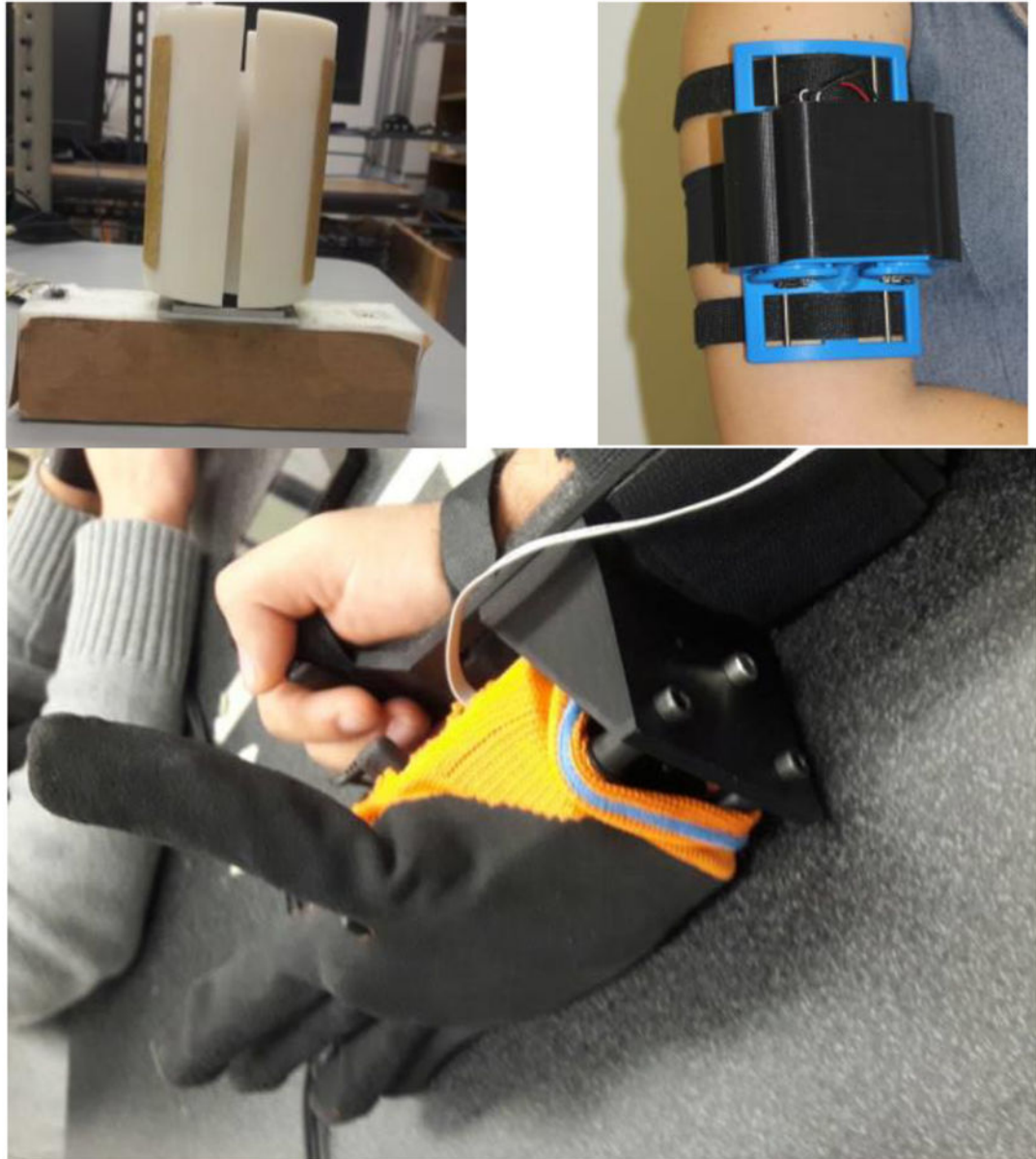
Figure 1. Clockwise from top left: the inverted-T sensorized object, the CUFF, and the SoftHand Pro with the forearm adapter.
