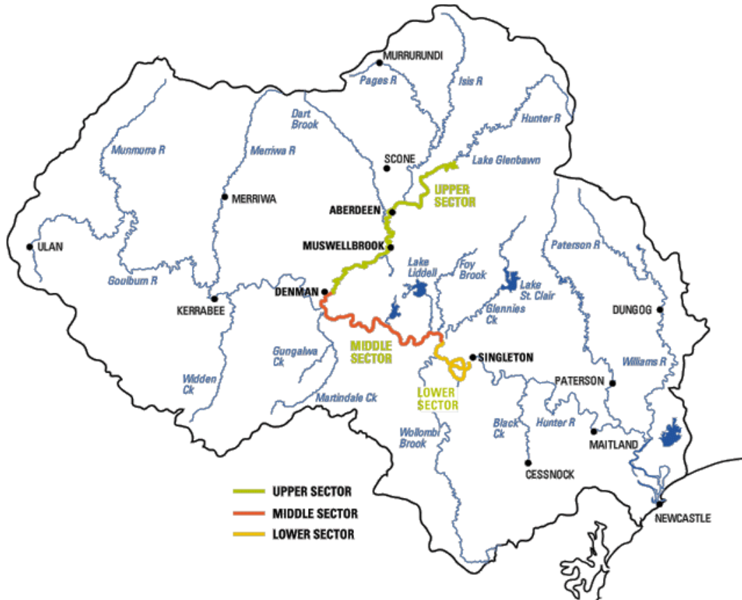
Figure 1. Map of the Hunter River Basin showing Hunter River and its major tributaries. The compliance monitoring station for salinity is located at Singleton where an EC of 900 uS/cm should be met 95% of the time. The Hunter River Basin salinity management project is one of the most innovative and successful projects of its type in the world. http://www.environment.nsw.gov.au/licensing/hrsts/allocating.htm
