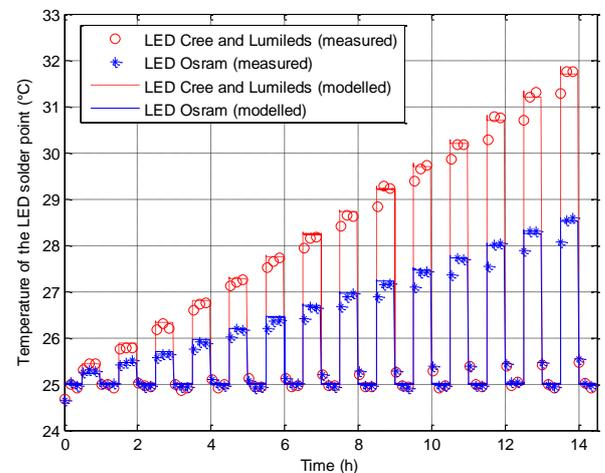
Fig. 9. Evolution of LED solder point temperatures
