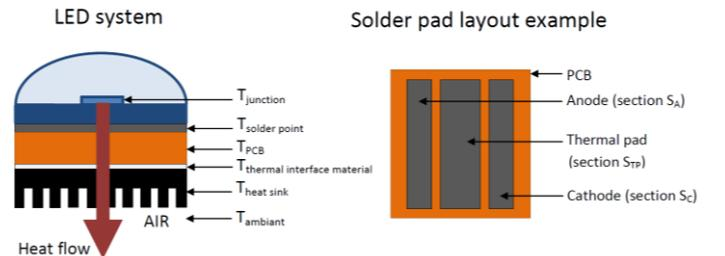
Fig. 6. Thermal variables used to model an LED system
