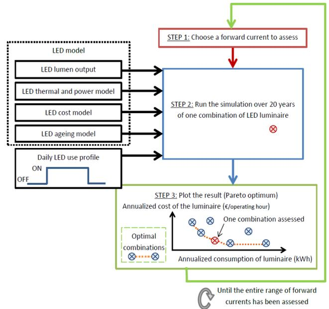
Fig. 2. Flowchart of the LED optimization methodology
