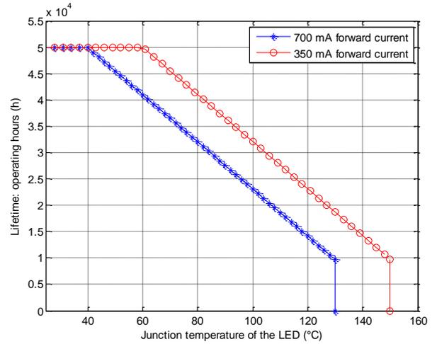
Fig. 10. Simplified lifetime model of an LED [26]
