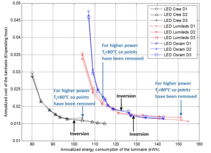
Fig. 11. Annualized cost vs. power of the luminaire
