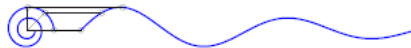
Figure 1: A damped oscillator in state space form. Left: At each time step, the state vector x rotates by \theta and its length becomes shorter. Right: The actual waveform is a one dimensional projection from the two dimensional state vector. The stochastic model assumes that there are two independent additive noise components that corrupt the state vector x and the sample y , so the resulting waveform y_{1:T} is a damped sinusoid with both phase and amplitude noise.
