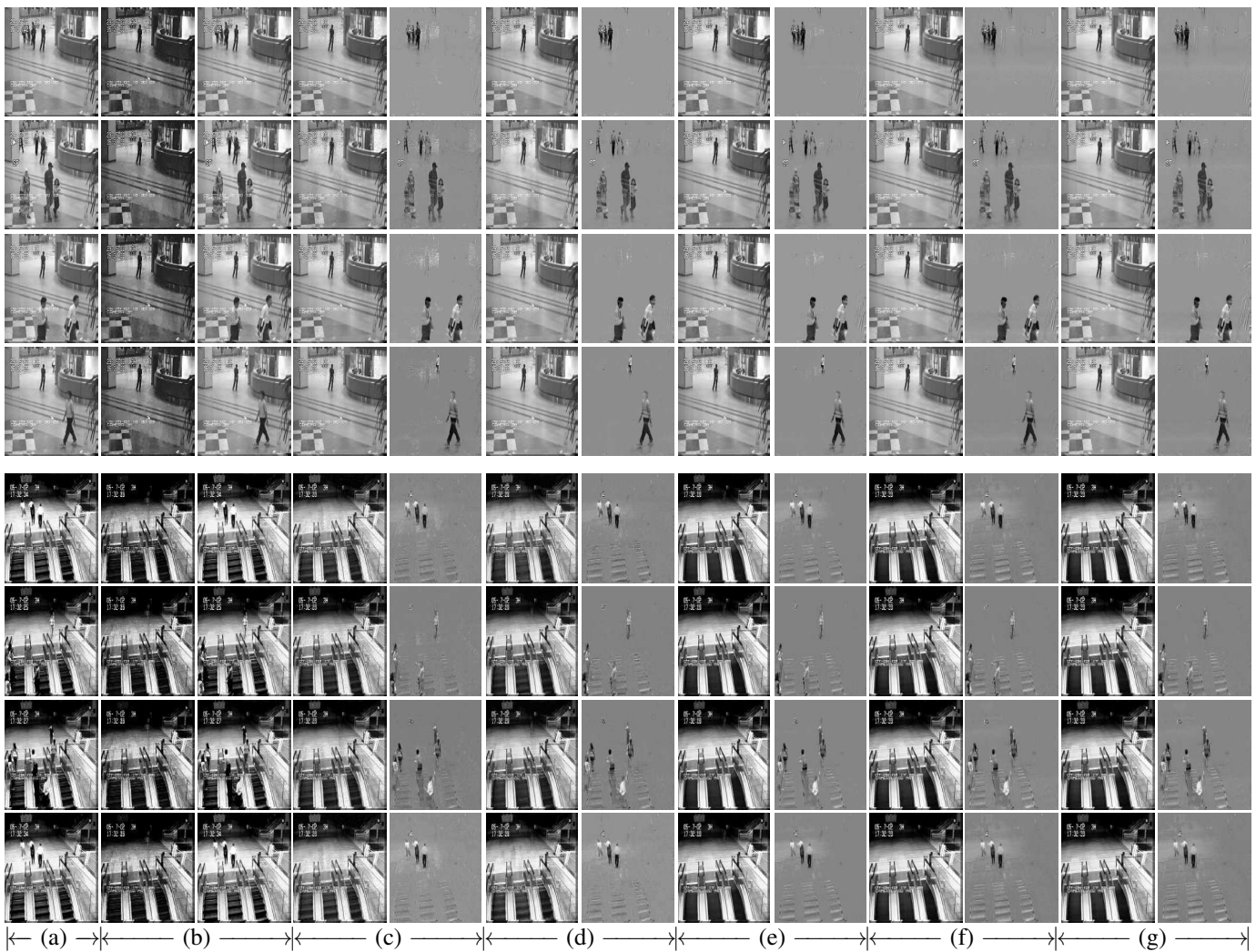
Fig. 9. Results of background-foreground separation by all the online and batch algorithms on the Hall (upper) and Escalator (lower) video sequences. The labels (a) to (g) denote the original video frames and results produced by ONMF, ORPCA, OADMM, OPGD, BADMM, BPGD respectively. For each algorithm, the left column denotes the background and the right column denotes the foreground (moving objects).
