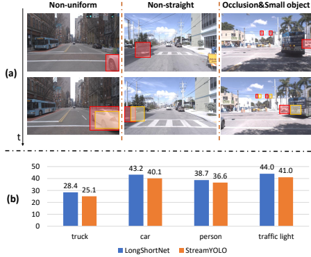
Fig. 2: (a) shows that StreamYOLO has suboptimal results, with red and orange boxes indicating ground truth and predictions. The comparison of sAP between LongShortNet and StreamYOLO is presented in (b). More examples can be found at https://rebrand.ly/wgtc1oo .
