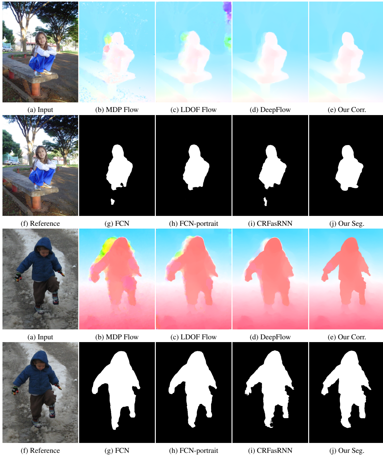
Figure 8. Visual comparisons of different segmentation and correspondence estimation methods. (a) and (f) are the input and reference images respectively. (b-e) are the correspondence estimated by MDP [49], LDOF [11] and DeepFlow [45] respectively. (g-i) are the FCN, FCN-portrait and CRFasCNN segmentation results respectively. (e) is our correspondence result and (f) is our segmentation result.
