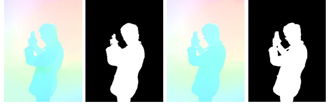
(a) Sep. Corr. (b) Sep. Seg. (c) Joint Corr. (d) Joint Seg. Figure 5. Comparison of separate and joint refinement on correspondence and segmentation using our CRF model. (a) and (b) are separately refined correspondence and segmentation results. (c) and (d) are the joint ones. The input is shown in Figure 4(a).
