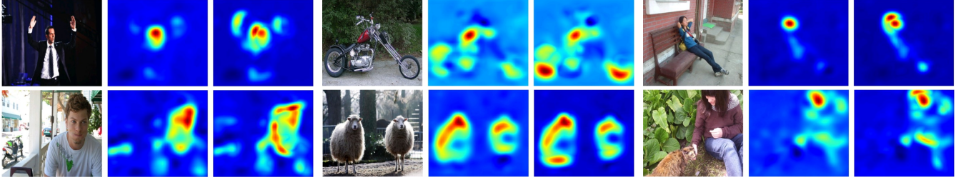
Figure 3: Object saliency detections using the first network (column 2, 5, and 8) and proposed method (column 3, 6, and 9).
