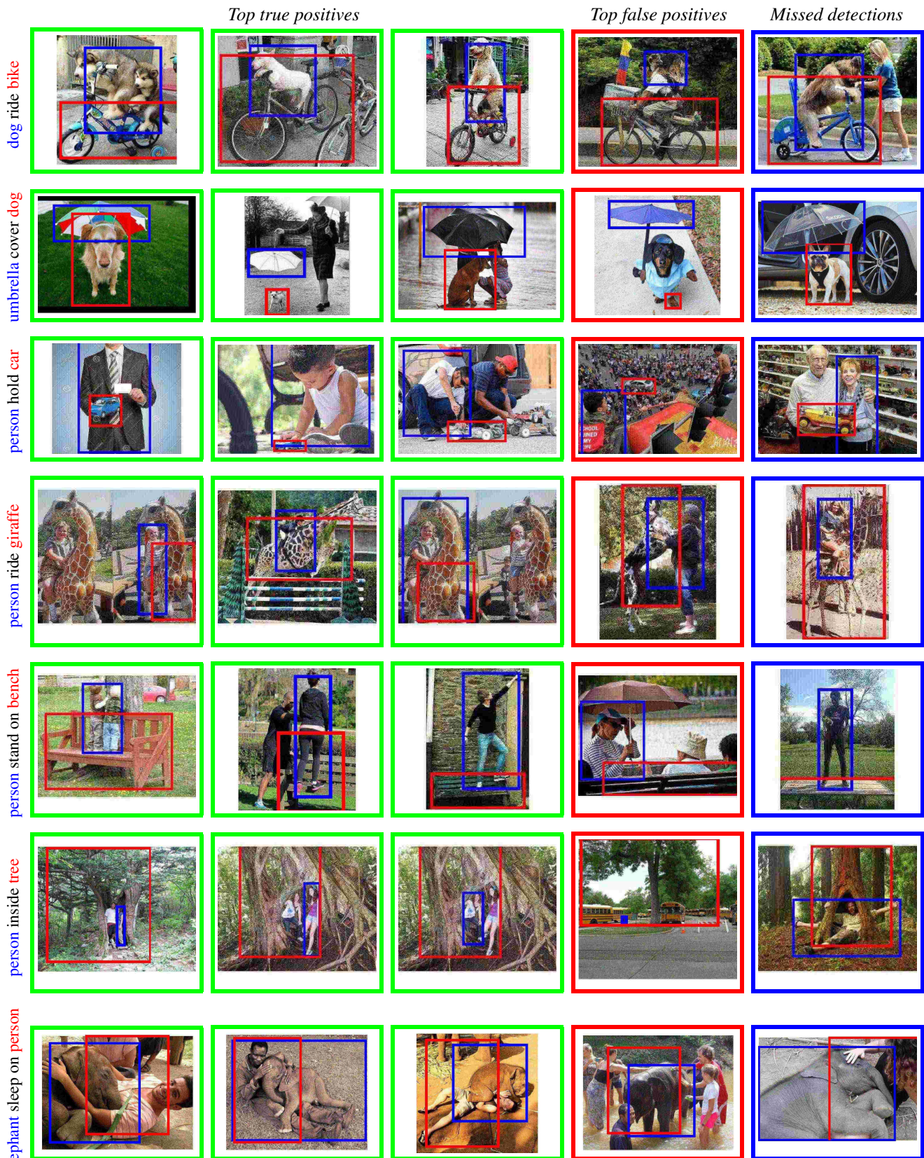
Figure 8: Examples of retrieved results for triplet queries on UnRel. Each row corresponds to one triplet query and displays true positives among the top-retrieved pairs (green), top-scored incorrect pairs (red) and missed detections (blue). These retrieval results were computed using our weakly-supervised method with candidate proposals. A pair of boxes is considered as positive if both subject and object candidates overlap with the corresponding subject and object ground truth with \text{IoU} \geq 0.3 .
