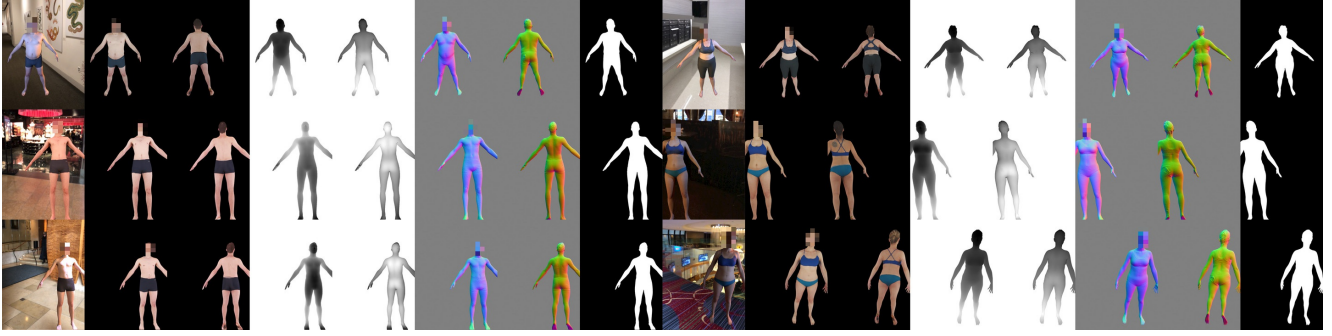
Figure 5: Each row shows two instances of synthetic data (one male, one female). For each example, left to right: RGB, front and back albedo, front and back depth, front and back normals, and segmentation. Note that these examples do not really belong to our training set, since the textures come only from test subjects who signed a special consent form.
