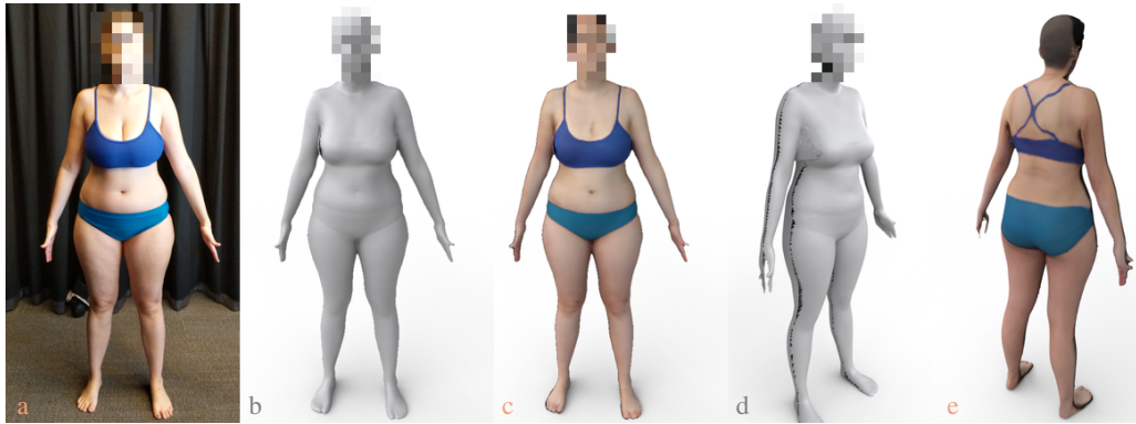
Figure 1: FAX converts a single RGB image (a) into a scan (b, d) with albedo texture (c, e)
