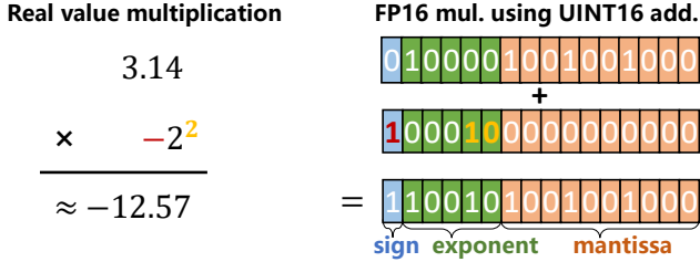
Figure 2: The multiplication between a float number and a positive or negative power-of-two integer can be implemented by an integer addition instruction, which allows DenseShift networks inference on most existing hardware efficiently. The FP16 dot-product computation achieved 1.6\times speed up on ARM A57 CPU using this technique as discussed in Sec. 3.1.1.
