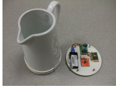
Fig. 2. A jug fitted with a CogWatch Instrumented Coaster (CIC) (left) and an ‘open’ CIC (right)
