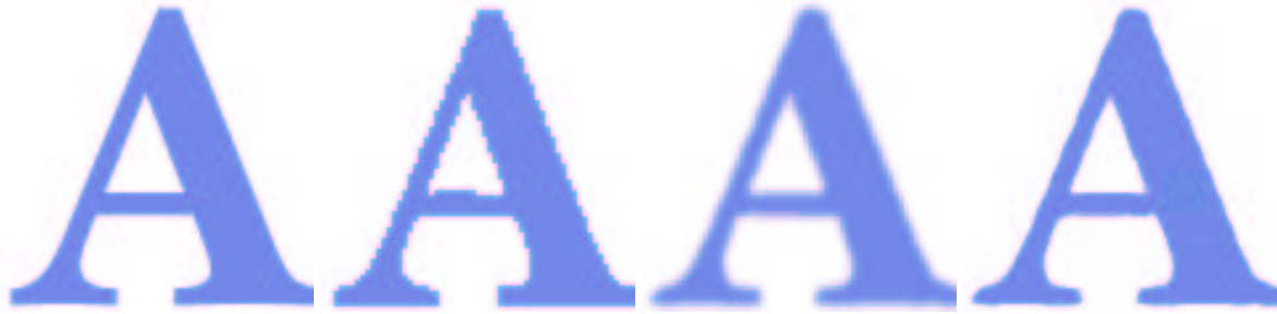
Fig. 3. Comparison of compression results. (a) A portion of the original 600dpi test image. Results of compression and decompression of a 300dpi original using (b) standard RDOS at 0.2014 bpp; (c) resolution enhanced rendering (RER) at 0.2016bpp; (d) resolution interpolated RER (IRER) at 0.2000 bpp.
