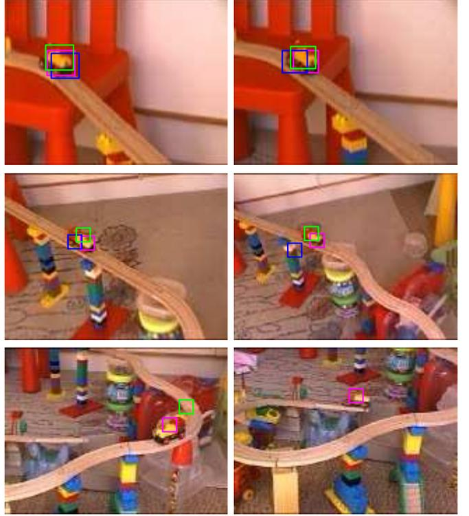
**Fig. 2.** Tracking result of proposed system (magenta) against SSD (green) and MS (blue) tracker for ‘train’ sequence. Frames shown 20, 50, 200, 270, 620 and 1150.
