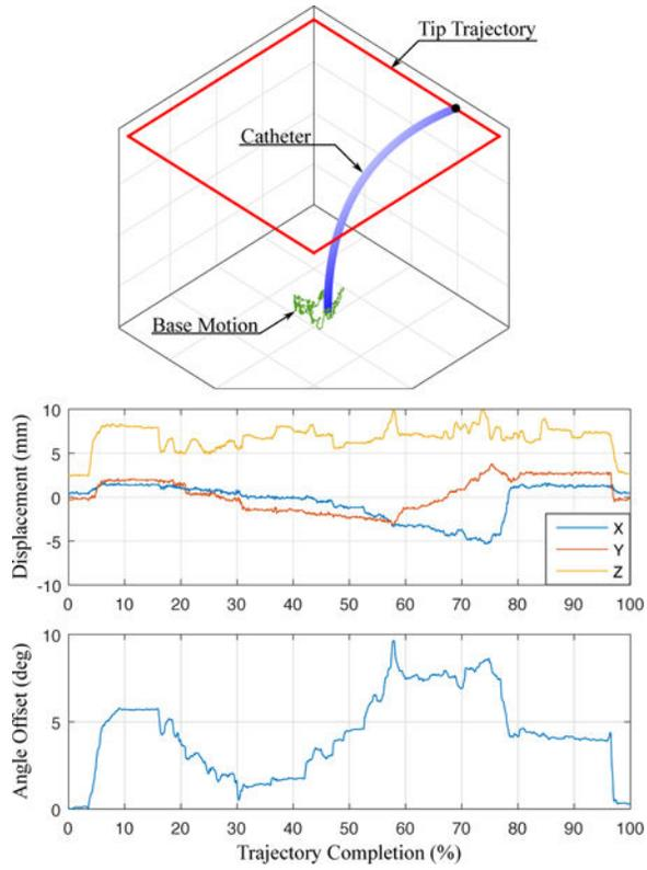
**Fig. 4.** Catheter navigation causes uncontrollable motion of the bending section base. (*top*) The base motion is measured (green) while the catheter tip is navigated along a square trajectory (red). (*middle*) The displacement of base point in *xyz* coordinates and (*bottom*) the change in base point rotation about the catheter axis are measured.
