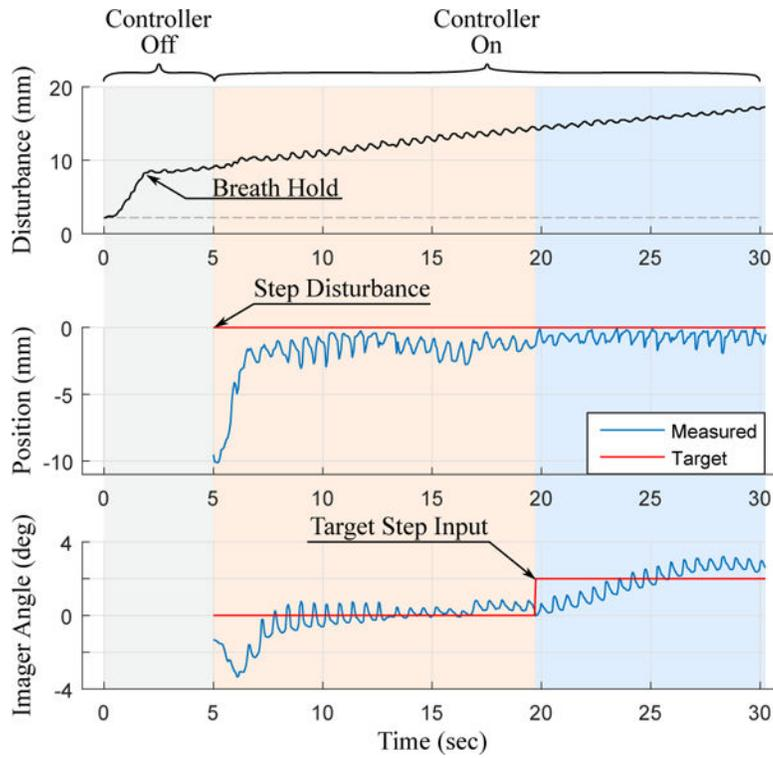
**Fig. 12.** *In vivo* tests demonstrating the ability of the robotic system to maintain the catheter tip at the target pose despite disturbance step, disturbance ramp, and target step inputs.
