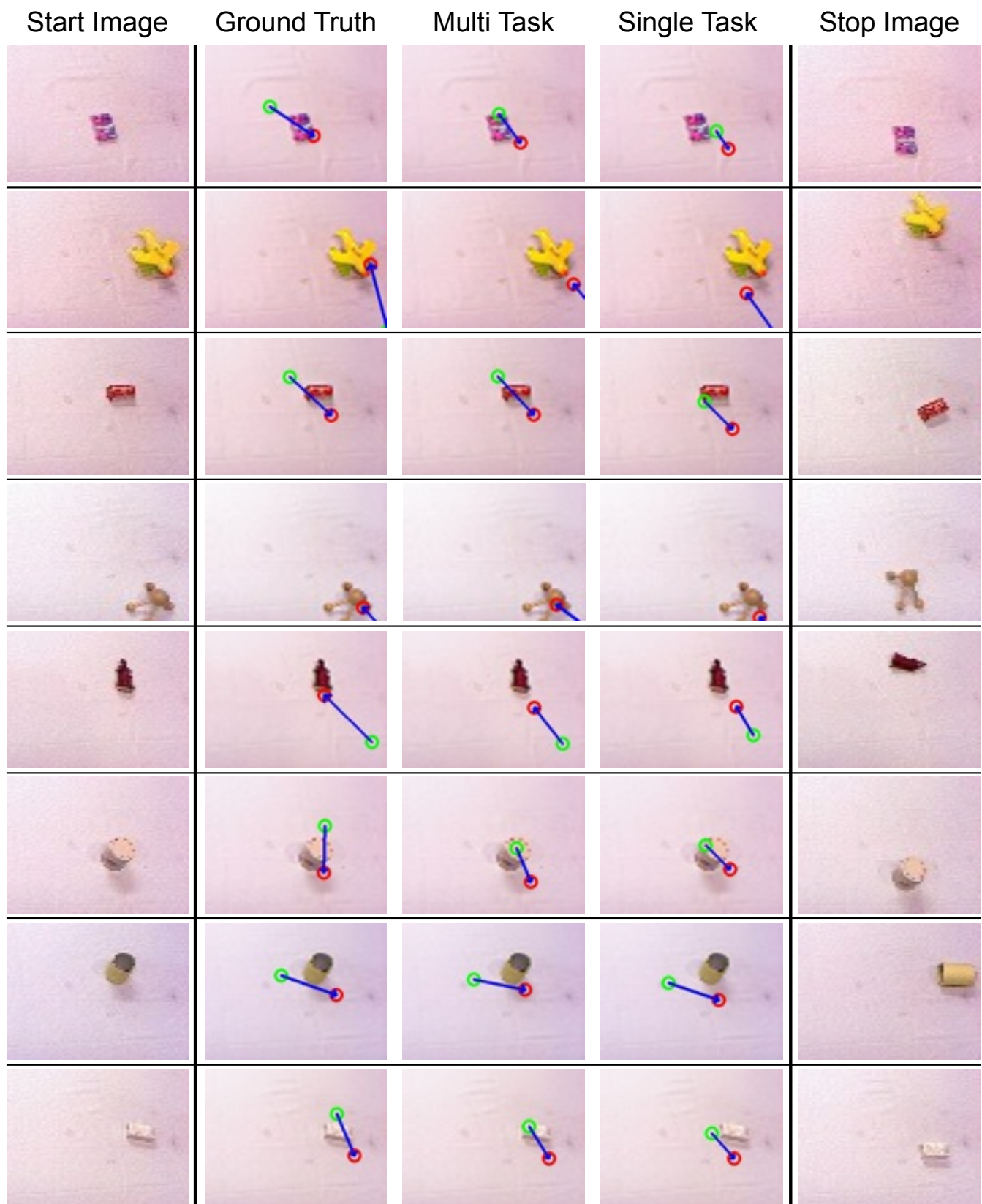
Fig. 9. We show the qualitative results for the pushing task, randomly sampled from the test set. The green circle represents the start configuration for the end effector, the red circle represents the final configuration of the end effector and the blue arrow represents the direction of push.
