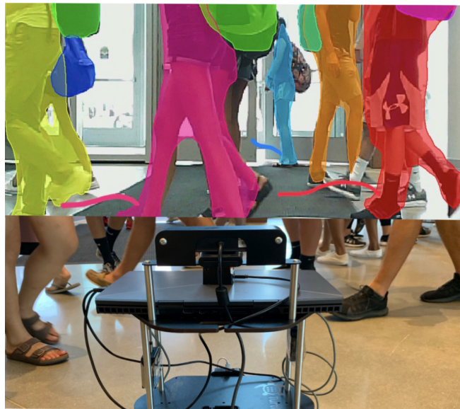
Fig. 1: We explicitly track and predict pedestrian motions (marked for the three pedestrians above) and use it to train a Deep Reinforcement learning-based collision avoidance policy. Our network implicitly learns to reduce the occurrence of the freezing robot problem and generates smooth robot trajectories in dense crowds.
