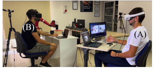
Fig. 6: Laboratory setting for the practical implementation of the Physical Metaverse. The user A pours the water in B's cup thanks to the Avatarm, while B observes the scene.
