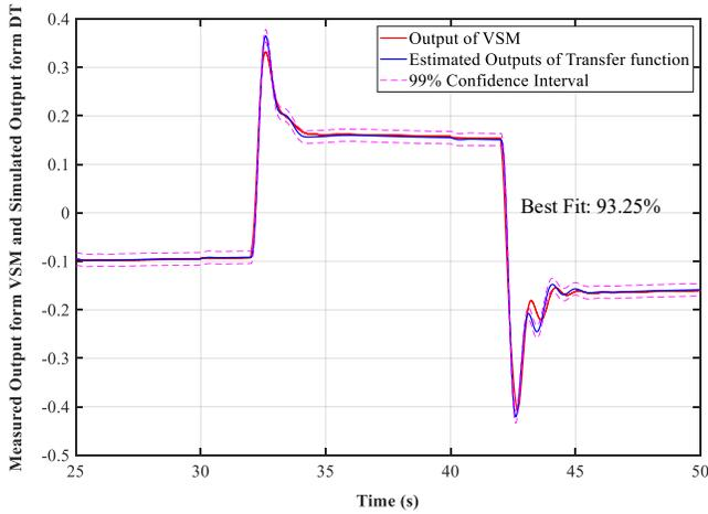
Fig. 7: Comparison between VSM and the corresponding transfer function
