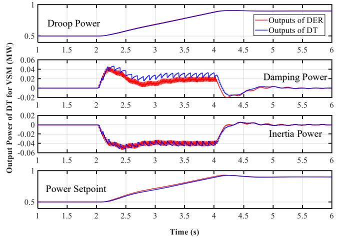
Fig. 9: The performance of DT in real-time monitoring with estimated minimum reporting rate (17 Hz)
