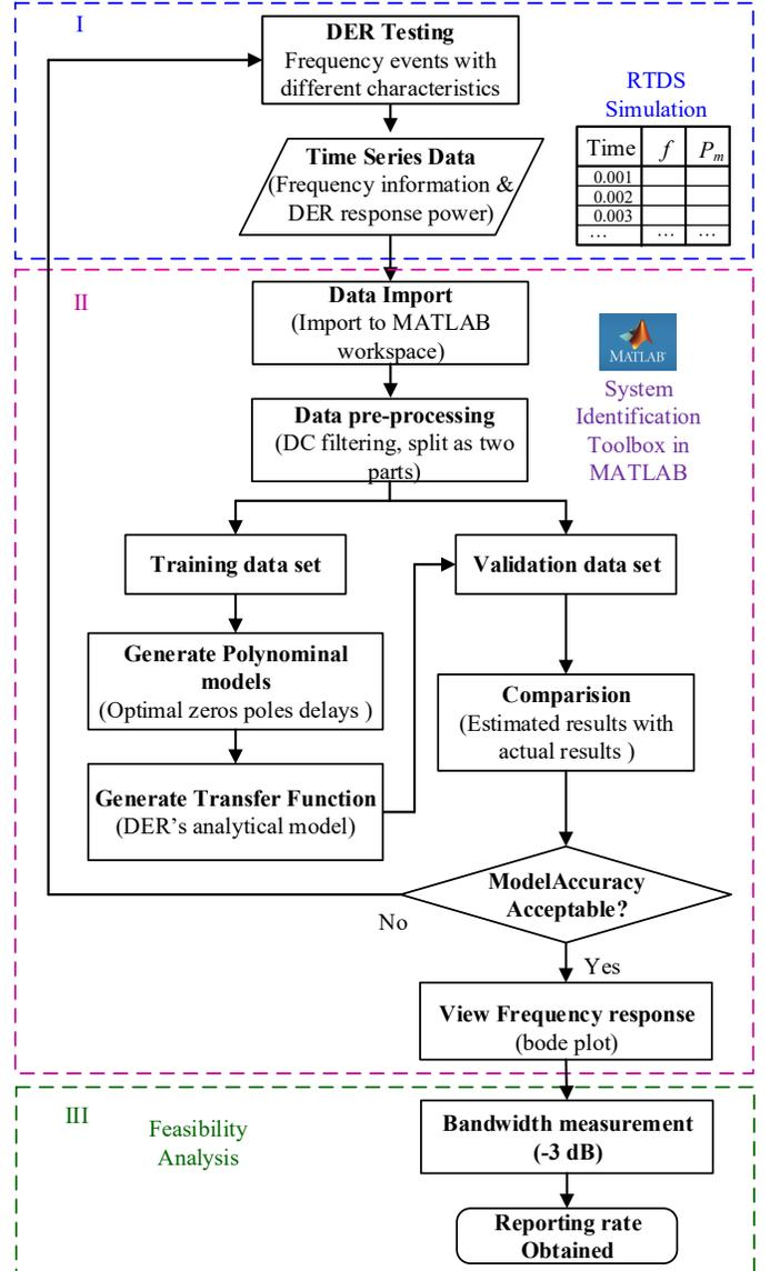
Fig. 6: Data-driven based frequency response analysis
