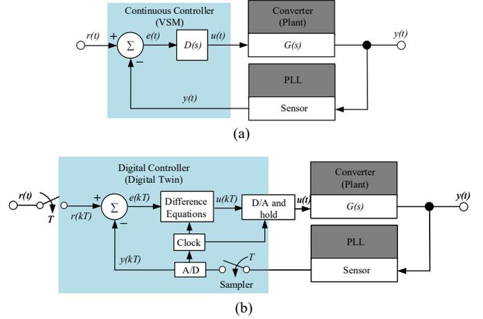
Fig. 2: Continuous controller to digital controller: (a) VSM (b) DT of VSM
