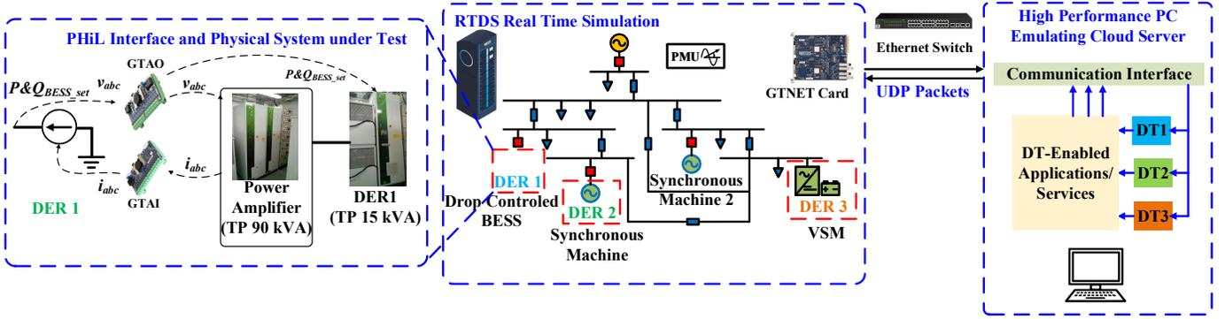
Fig. 5: Experimental platform to validate the effectiveness of the proposed reporting rate selection methods.
