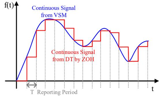
Fig. 3: Discretization of DT model by ZOH method.
