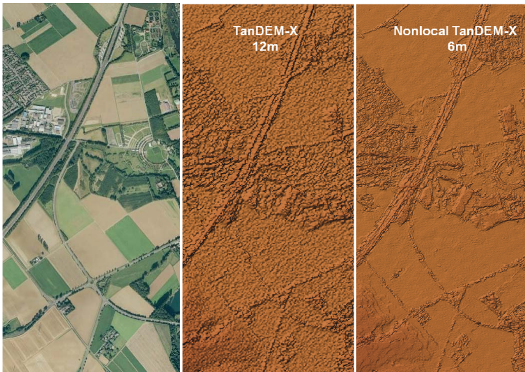
Fig 4: Jülich city area: Optical image ©Google (left), standard TanDEM-X DEM (middle) and improved nonlocal TanDEM-X DEM (right).
