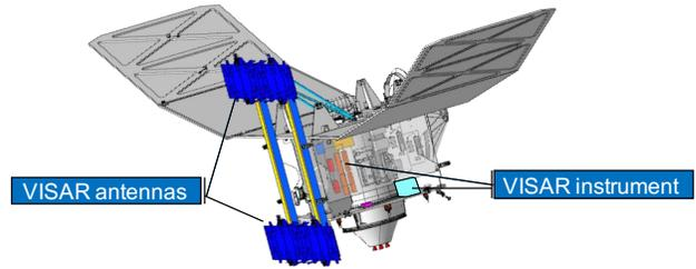
**Fig. 1:** The VERITAS spacecraft with its two VISAR antennas and the instrument [1, 2, 3].
