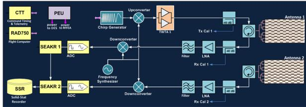
**Fig. 2:** VISAR instrument functional block diagram.
