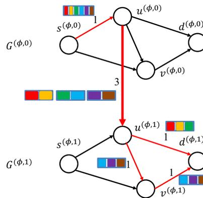
Fig. 8. Micro packets in an efficient route. The sizes of a micro packet on a link in  $\mathcal{G}^{(\phi,0)}$ , link  $(u^{(\phi,0)}, u^{(\phi,1)})$ , and a link in  $\mathcal{G}^{(\phi,1)}$  are  $1/6$ ,  $1/2$ , and  $1/3$ , respectively. Scaling factors:  $x^{(\phi,1)} = 3$ ;  $w^{(\phi,1)} = 2$ .
