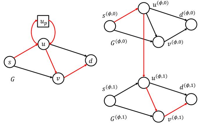
Fig. 2. The left figure is the original graph  $\mathcal{G}$ , where  $u$  is the only computation node for the single function in  $\phi$ . A dummy node  $u_p$  and connections to  $u$  are added to illustrate the availability of service function processing at node  $u$ . The right figure is the layered graph  $\mathcal{G}^{(\phi)}$ .
