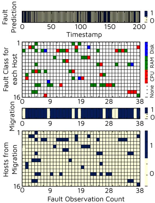
Figure 4: Visualization of fault prediction, classification and migration decisions with execution intervals.
