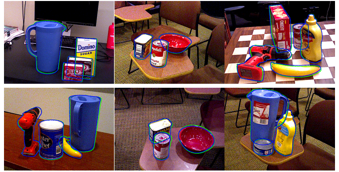
Fig. 8. Qualitative results on YCB-Video dataset [6]. Ground truth and predicted object poses are visualized as object contours in green and blue colors, respectively.
