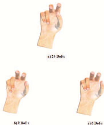
(b) Prismatic grasping reconstruction. a)Original Gesture b)Hand model reconstructed by 9 elements c)Hand Model reconstructed by 6 elements
