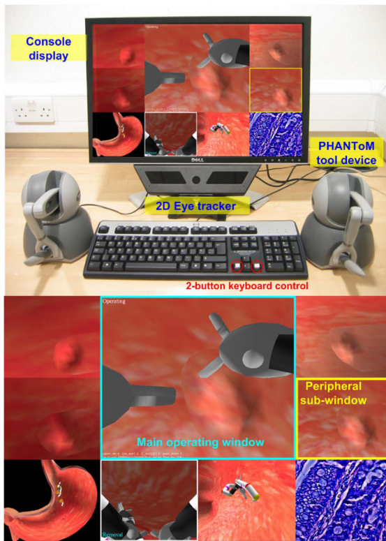
Fig. 1. Top: The overall setup of the control environment including two PHANToM Omni tool devices and a Tobii eye tracker. Bottom: A snapshot of the console display.
