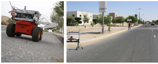
Fig. 6: The stereo camera mounted on a mobile robot (left), and the length of road used for dataset collection (right).
