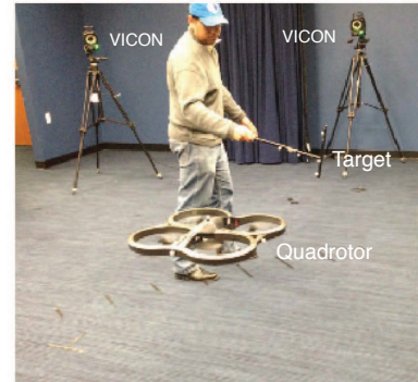
Fig. 5. Experimental setup : reflective markers were used to track the target and locate the Parrot quadcopter with the VICON motion capture system.
