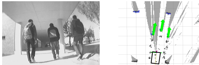
Fig. 6. (a) Image from a wide-angle camera. (b) Representation of the laser measurements, showing the three tracked subjects and their orientation as the green vectors, the robot is represented as the black rectangle.
