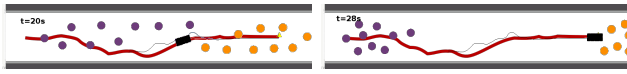
Fig. 2. Navigation using A* motion planning. Due to the motion of agents, the algorithm is constantly replanning, hindering the robot motion.
