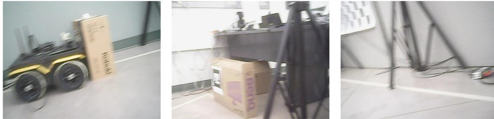
Fig. 11: Motion blurred frames
