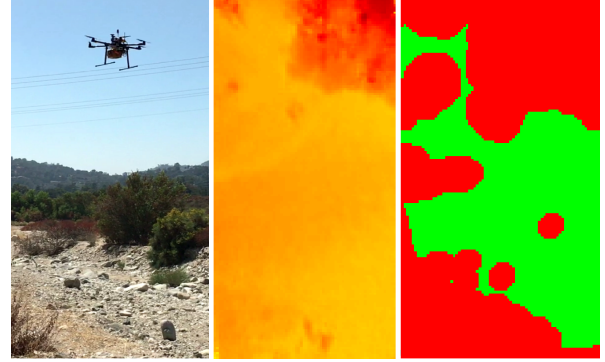
Fig. 1. UAV flight in outdoor environment. Middle: Top-down view of color-coded elevation map (warmer colors are closer to the camera); Right: Associated landing site map (Green: safe landing sites, Red: hazards).
